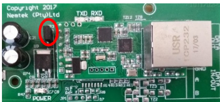
8-Way Relay Board JP3 Ensure jumper installed on the 2 upper pins as in the figure.
